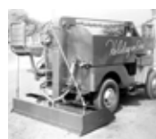
Zamboni #12 for Holiday on Ice. The stepped underside of the snow tank in the front was unique to #12 and #14.
